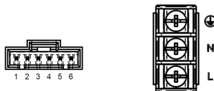
Figure 3 - LPM616 Front Panel Connectors Pinout View
